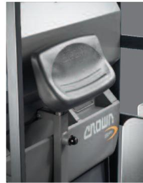
**Backrest** for Load-Facing Operator Controls
