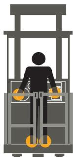
**Four points of solid contact on the SP 3500 Series,** with right-hand fixed control, enhance operator stability and confidence at height.
